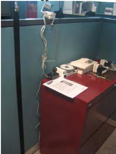
Figure 6. Temperature and humidity data logger installation.
